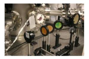
Mirrors are used in scientist Mark Tillack's UC San Diego photonics lab to guide light into laser amplifiers.
