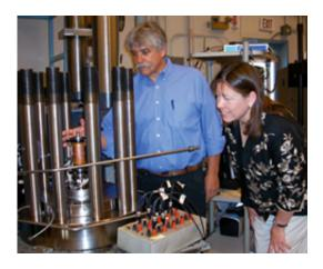
Sandia researchers Steve Bauer and Georgianne Peek look at equipment that will be used to analyze core samples from the potential Iowa aquifer compressed air energy storage site. The data will provide necessary fundamental information used for the design and performance of the underground air storage vessel. (Photo by Chris Burroughs)
