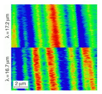
False color image of the electric domains on the surface of a bariumtitanate crystal. Image (a) was measured with a wavelength of 17.2 micrometers, image (b) of 16.7 micrometers. The color red means a strong signal. The change of the colors from red to blue is clearly visible.
