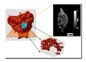
Section and isosurface rendering of a 500 nm cube from the interior of the 3D volume. The foam structure shows globular nodes that are interconnected by thin beam-like struts. Approximately 85% of the total mass is associated with the nodes, and there is no evidence of asignificant fraction of dangling fragments.
