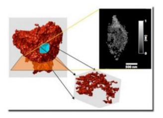
Section and isosurface rendering of a 500 nm cube from the interior of the 3D volume. The foam structure shows globular nodes that are interconnected by thin beam-like struts. Approximately 85% of the total mass is associated with the nodes, and there is no evidence of asignificant fraction of dangling fragments.
