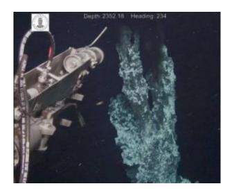
The top three feet of a chimney nearly 40 feet tall are visible as the arm of a remotely operated vehicle reaches in to sample fluids. The vent is part of the northernmost hydrothermal vent field yet seen and sampled. Credit: Centre for Geobiology/U. of Bergen
