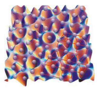
Particles in quasicrystalline light field: Stuttgart-based physicists superimposed five laser beams to create a quasicrystalline structure. Upon variation of the laser intensity the small plastic spheres arrange differently. At certain light intensities they form a pattern, shown here with red lines, similar to an ancient model - an Archimedean tiling. Image: Ingrid Schofron (MPI of Metals Research) & Jules Mikhael (University of Stuttgart)
