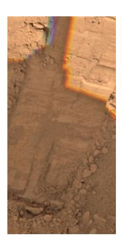
This image, taken by NASA's Phoenix Mars Lander's Surface Stereo Imager on Sol 50, or the 50th day of the mission, July 15, 2008, shows two holes at the top created by the lander's Robotic Arm's motorized rasp tool. Image: NASA
