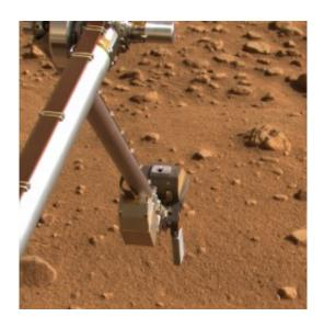
This image taken by the Surface Stereo Imager on Sol 49, or the 49th Martian day of the mission (July 14, 2008), shows the silver colored rasp protruding from NASA's Phoenix Mars Lander's Robotic Arm scoop. The scoop is inverted and the rasp is pointing up. Shown with its forks pointing toward the ground is the thermal and electrical conductivity probe, at the lower right. The Robotic Arm Camera is pointed toward the ground. (NASA/JPL-Caltech/University of Arizona/Texas A&M University)
