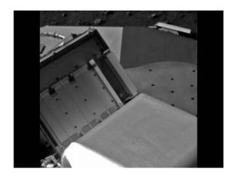
The double doors on the right are wide open in this image of four pairs of oven doors on Phoenix's Thermal and Evolved-Gas Analyzer (TEGA). Image credit: NASA/JPL-Caltech/University of Arizona/Texas A&M University
