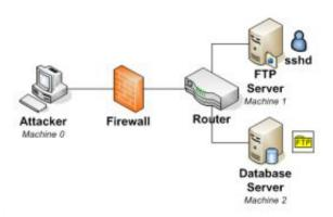
The example illustrates three paths that an attacker can take to penetrate the network using FTP server, SSH server or database server. Image: NIST
