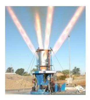
A full-scale rocket motor fires from the Aerojet facility in Sacramento, Calif. This test will help in the development of NASA's Orion jettison motor that is being designed to separate the spacecraft's launch abort system from the crew module during launch. (Aerojet)
