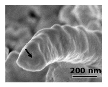
A scanning electron microscope image of a cross section of a GeTe/Ge<sub>2</sub>Sb<sub>2</sub>Te<sub>5</sub> nanowire (the arrow points to the Ge<sub>2</sub>Sb<sub>2</sub>Te<sub>5</sub> core).
