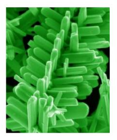
Researchers have discovered a new method to create branched nanorods, such as those in this scanning electron microscope image. Such nanorods could one day enable new nanoscale thermoelectric devices for power generation, as well as nanoscale heat pumps for cooling hot spots in nanoelectronics devices. Image: Rensselaer/Ramanath
