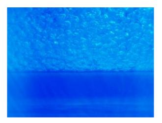
Nanoparticle additives to lubricants commonly combined with refrigerants used in chillers may encourage secondary nucleation-bubbles on top of bubbles. The double-bubble effect enhances boiling heat transfer and, ultimately, could help to boost the energy efficiency of industrial-sized cooling systems. Image: NIST
