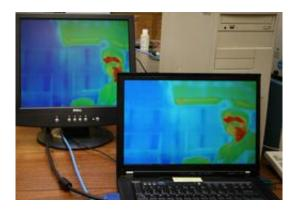
Thermal images are displayed on a computer screen via an infrared camera which detects the presence of hard objects inside camouflaged boxes.
