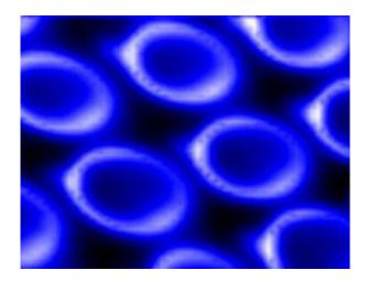
Image of an array of microscopic magnets taken with scanned probe ferromagnetic resonance force microscopy -- a new imaging technique invented by Ohio State University physicists and colleagues. The disk-shaped magnets measure only two micrometers (millionths of a meter) across. Image courtesy of Ohio State University.
