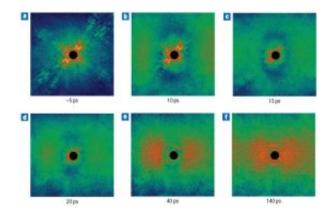
Soft X-rays from the FLASH laser capture the action as a tiny silicon nitride wafer explodes.
