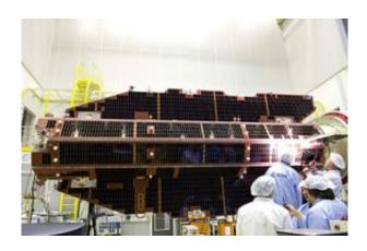
Solar panel inspection during final testing at ESA-ESTEC. Credits: ESA
