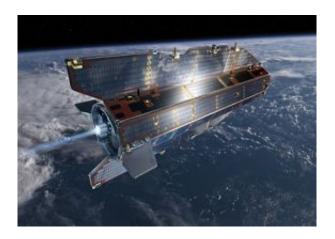
In orbit, the same side of the GOCE satellite remains facing the Sun. The spacecraft is equipped with four body-mounted and two wing-mounted solar panels. Due to the configuration in orbit, the solar panels will experience extreme temperature variations so it has been necessary to use materials that will tolerate temperatures as high as 160°C and as low as -170°C. Credits: ESA -AOES Medialab
