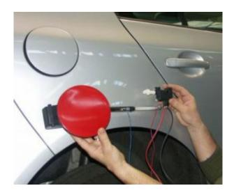
The fuel filler flap will be released by a single wire instead of a small servo motor in future. Credit: Fraunhofer IWU
