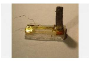
This torque cantilever is used to measure magnetic property of bismuth in intense magnetic fields. The bismuth crystal (5.6 mm tall vertical pillar) is glued to the end of a thin cantilever beam made of gold. Deflections of the cantilever in a field are detected by measuring changes in capacitance. Credit: N. Phuan Ong, Princeton University
