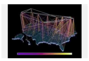
This image is a visualization study of inbound traffic measured in billions of bytes on the NSFNET T1 backbone for the month of September 1991. The traffic volume range is depicted from purple (zero bytes) to white (100 billion bytes). It represents data collected by Merit Network, Inc. Credit: Donna Cox and Robert Patterson, courtesy of the National Center for Supercomputing Applications (NCSA) and the Board of Trustees of the University of Illinois
