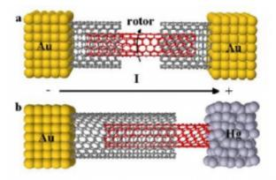
The proposed (a) nanomotor and (b) nanodrill, where the red inner CNT rotates due to an electron wind. The nanomotor is attached to gold electrodes, which act as electron reservoirs, while the nanodrill has one end contacted to a mercury electrode. Credit: S.W.D. Bailey, et al.
