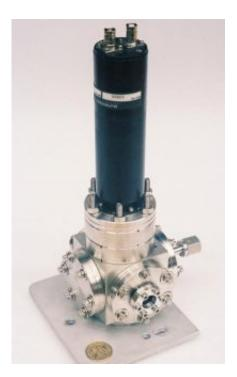
NIST Lyman alpha neutron detector, shown with a US dollar coin for scale, is now the world's most sensitive neutron detector. Credit: NIST
