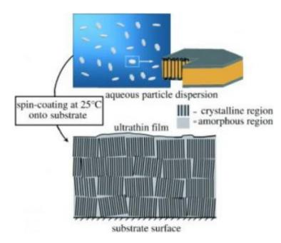
Caught on film: Ultrathin (50 nm) films of crystalline polyethylene were prepared at room temperature from prefabricated polymer nanocrystals functioning as building blocks. The very small particle size, in combination with the phenomenon that the amorphous regions are located at the surface exclusively in polymer single crystals, results in efficient interaction between particles in the films. Credit: (C) Wiley-VCH 2008
