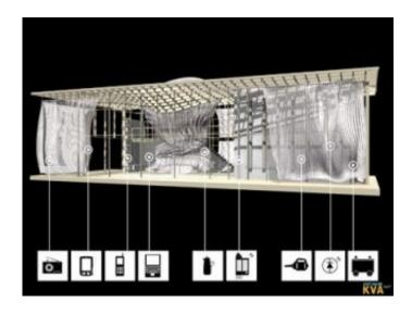
A 3-D rendering of "Soft House", which uses household curtains to collect solar energy and provide lighting.
