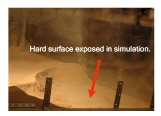
University of Michigan simulations performed with crushed walnut shells at NASA's Ames Research Center show that Mars Phoenix thrusters would strip loose soil to the hard surface.
