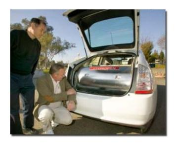
Salvador Aceves (left) and Tim Ross check out the on-board hydrogen storage tank that powers a prototype hybrid vehicle. Photos by Jacqueline McBride/LLNL
