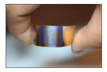
An array of printed transistors on plastic.
