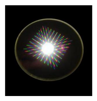
Caption: Microscopic magnets (above left), designed and tested in a joint NIST/NIH project, might one day be injected into the body to add color and "smart tag" capability to magnetic resonance imaging for medical diagnosis and research. The image on the right shows light scattering from grids of magnets on a wafer where they were made using conventional microfabrication techniques. (RIGHT IMAGE) Credit: G. Zabow, NIST/NIH
