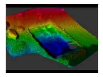
This color-coded elevation map shows the "Dodo-Goldilocks" trench dug by the Robotic Arm on NASA's Phoenix Mars Lander. Image credit: NASA/JPL-Caltech/University of Arizona/Texas A&M University/NASA Ames Research Center
