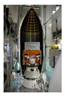
The first half of the payload fairing is moved into place around NASA's Gamma-Ray Large Area Space Telescope within the mobile service tower on Launch Pad 17-B at Cape Canaveral Air Force Station. The fairing is a molded structure that fits flush with the outside surface of the Delta II upper stage booster and forms an aerodynamically smooth nose cone, protecting the spacecraft during launch and ascent. Photo credit: NASA/Jim Grossmann
