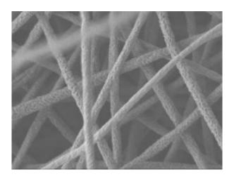
Scientists report development of a plastic that is 10 times more stretchable than that of the original material. Above is a micrograph of the electrospun nano-sized fibers. Credit: Courtesy of the American Chemical Society
