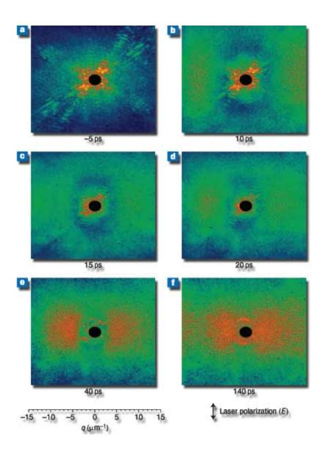
Sample evolution revealed by coherent X-ray diffraction. Measured single-shot diffraction patterns at 25 ps (a ), corresponding to the object just before the laser excitation pulse, and diffraction patterns from the same object at 10 ps (b), 15 ps
