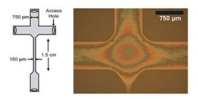
Left: Schematic of a T-junction nanofluidic device with a "nanoglassblown" funnel-shaped entrance to a nanochannel. The funnel tapers down to 150 micrometers (about the diameter of a human hair) at the nanochannel entrance. Right: Photomicrograph of the T-junction with the first section of the nanochannel visible at the bottom. The colors are a white light interference pattern caused by the changing depth of the curved glass funnel. Credit: Elizabeth Strychalski, Cornell University
