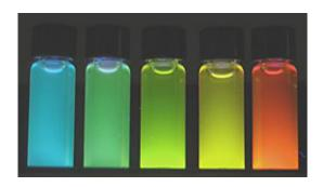
Brightly glowing vials of highly luminescent, water soluble quantum dots produced by the new NIST microwave process span a wavelength range from 500 to 600 nm. Credit: NIST
