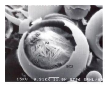
SRNL researchers removed the top of a glass microsphere to show how palladium has easily passed through the sphere's pores and assembled itself into a new nanostructure. Credit: Savannah River National Lab, American Ceramic Society
