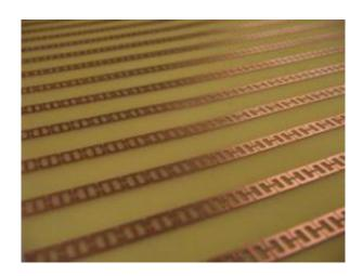
Researchers have engineered a metamaterial that uses tiny geometric surface features to successfully capture the electric and magnetic properties of a microwave to the point of total absorption. Image courtesy of Boston College
