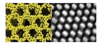
Computer simulation, left, shows how platinum nanoparticles will fuse into a structure with tiny pores after the polymers that guide them into position are removed. Right, electron microscope photo of the actual structure.
