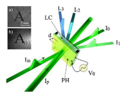
When a weak intensity and high intensity beam are aimed at a liquid crystal valve, the output pulse is split into different diffracted pulses, each showing a different group velocity. The images at left demonstrate image delay: image (a) is an original image imposed on the input pulse, and image (b) is the image from an output pulse delayed by several milliseconds. Credit: S. Residori, et al.
