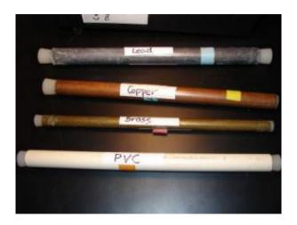
Plumbing systems with polyvinyl chloride plastic pipes could be more susceptible than copper pipes to leaching of lead and copper into drinking water, researchers report. Credit: Courtesy of Marc Edwards
