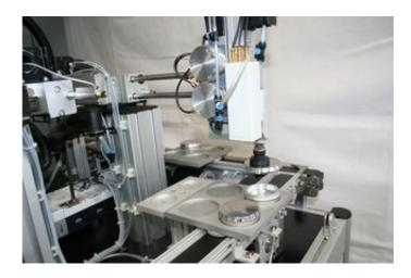
The demonstrator – a miniature conveyer system driven by compressed air – contains wireless sensors that provide their own power supply. © Festo
