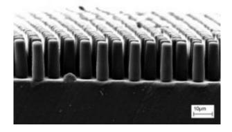
The sensor is covered with 250,000 tiny plastic columns only five microns in diameter. When a cell creeps across the tips of the columns, it presses each column very slightly sideways. Credit: © Fraunhofer IFAM
