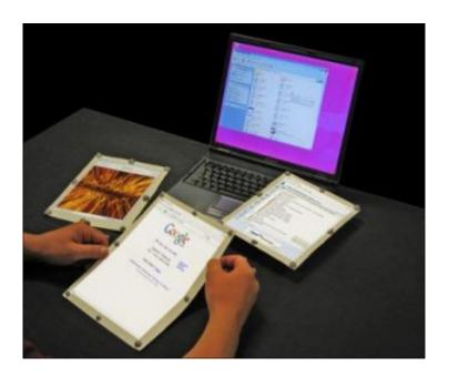
A prototype paper computer developed in Queen's Human Media Laboratory uses leaf turns to navigate documents. Credit: Queen's University Human Media Laboratory
