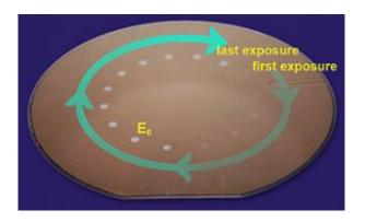
NIST researchers exposed a 300 mm silicon wafer with incrementally increasing doses of extreme ultraviolet light (EUV) in 15 areas. After the wafer was developed, the team determined that the seventh exposure was the minimum dose required (E0) to fully remove the resist. Credit: NIST
