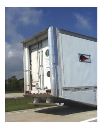
Aerodynamic improvements on truck trailers—such as rounded corners—coupled with pneumatic controls for blowing air from slots, help reduce drag and improve fuel economy for heavy trucks.
