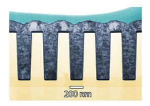
Working in the trenches: Transmission electron microscopy image of a thin cross section of 160 nanometer trenches shows deposited nickel completely filling the features without voids. (Color added for clarity.) Credit: NIST
