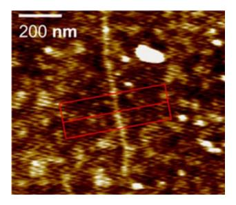
This atomic force microscope image shows a single-walled CNT with a height of 0.8 nm and length of 800 nm. Researchers found that, under low temperatures, CNTs emit one photon at a time, marking the first demonstration of nonclassical optical emission from a CNT. Credit: Högele, Alexander, et al.
