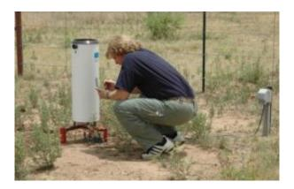
Dr. Brent Auvermann, Texas AgriLife Research engineer in Amarillo, downloads rainfall data from an electronic rain gauge used to calculate wet deposition as a part of the National Atmospheric Deposition Program. Credit: Texas AgriLife Research photo by Kay Ledbetter
