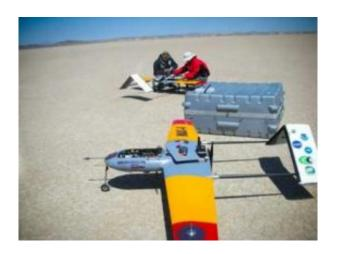
Technicians prepare an autonomous unmanned aircraft for launch at Edwards Air Force Base. The The Scripps-led California AUAV Air Pollution Profiling Study (CAPPS) used unmanned aircraft to make several types of meteorological measurements in the atmosphere. Data from CAPPS helped researchers characterize Southern California's smog and identify its many points of origin. Credit: Scripps Institution of Oceanography, UC San Diego
